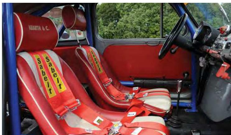
Dogleg first is down and to the left. Is it in? No. Try again. Still no. Lift the clutch pedal slightly and the lever now has a chance to engage. This is a technique I recognise from my Moto Guzzi-engined motorbike-gearbox Triking; you just have to crunch and bear it.
